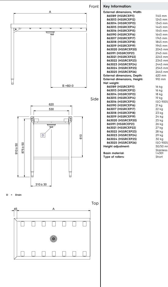
1945 mm 2045 mm 2145 mm 2245 mm 2345 mm 2445 mm 2545 mm 2645 mm 620 mm 910 mm 16 kg 16 kg 18 kg 19 kg ISO 9001; ISO 14001 kg 21 kg 22 kg 23 kg 24 kg 25 kg 26 kg 27 kg 28 kg 29 kg 30 kg ISO 9001; ISO 14001 kg 50/50 mm Stainless Steel AISI 304 - EN 1.4301 Short
